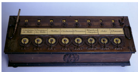
The Pascaline or Pascal's Calculator, by Blaise Pascal. It could add, subtract, multiply and divide two numbers (1642)
